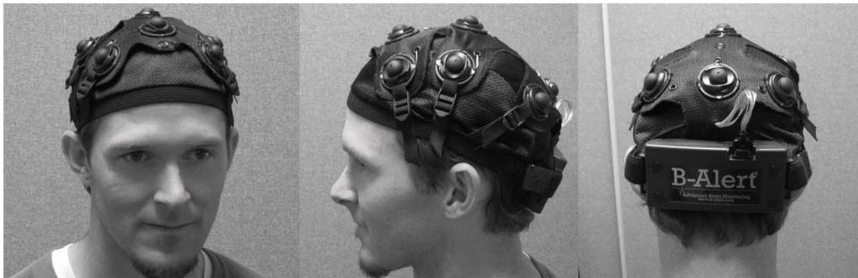
Figure 2: Wireless sensor headset
